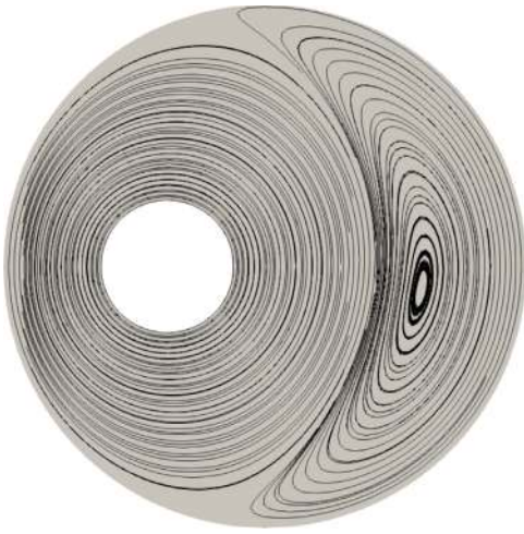
Fig. 14. Streamlines for the eccentric Couette flow (with \xi = 0.5 ) at the steady state obtained using Solver V.
